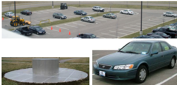
Figure 2: Optical images of parking lot being imaged in GOTCHA dataset, [18]. The scene contains a variety of calibration targets, such as primitive reflectors like the tophat shown, a Toyota Camry, forklift, and tractor.
