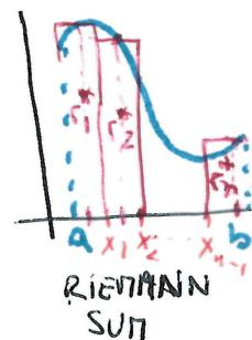
STEP 1: Pick  $a = x_0 < x_1 < \dots < x_{n-1} < x_n = b$  and  $\Delta x_k = x_k - x_{k-1}$  for  $k=0, 1, \dots, n$
