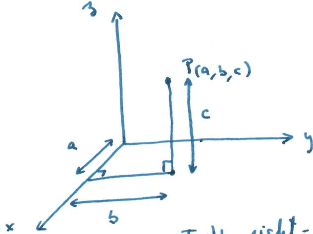
Note: The coordinate axes are directed according to the right-hand rule
