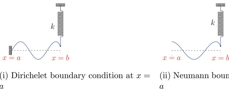
Figure 1.4: Vibrating strings each with a spring at one side and fixed (i) or free (ii) boundary condition at the other
