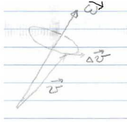
Figure 5.11: Vectorial change \Delta \vec{v} in \vec{v} due to its rotation around \vec{\omega} . The tip of \vec{v} moves in a plane perpendicular to \vec{\omega} and the tip's angle of rotation during time interval \Delta t is |\vec{\omega}|\Delta t .
