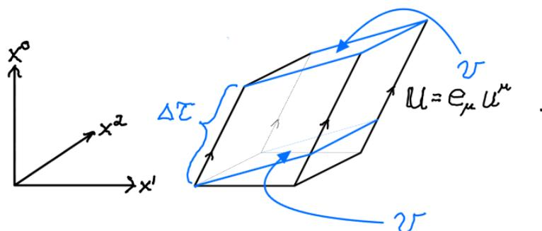
Figure 16.1 : World tube bounded by and filled with congruent particle world lines. The 4-d basis invariant spacetime volume  $\Delta\tau v$  is the product of the elapsed proper time  $\Delta\tau$  in a comoving element of fluid whose comoving volume is  $v$ .
