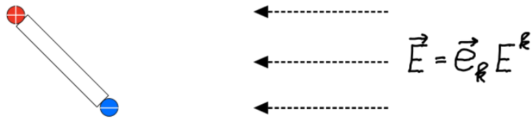
Figure 27.1 Macroscopic dipole in an electric force field.
