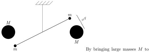
each of the masses m, Cavendish measured the gravitational force  $F_r$  by measuring the angular deflection of the pendulum.
