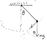
Since F = ma and S''(t) of the distance of arc = acceleration = 20''(t) which is equal to the a on the other side of the equal 9 sin 0, the component of acceleration of the force done by gravity.
