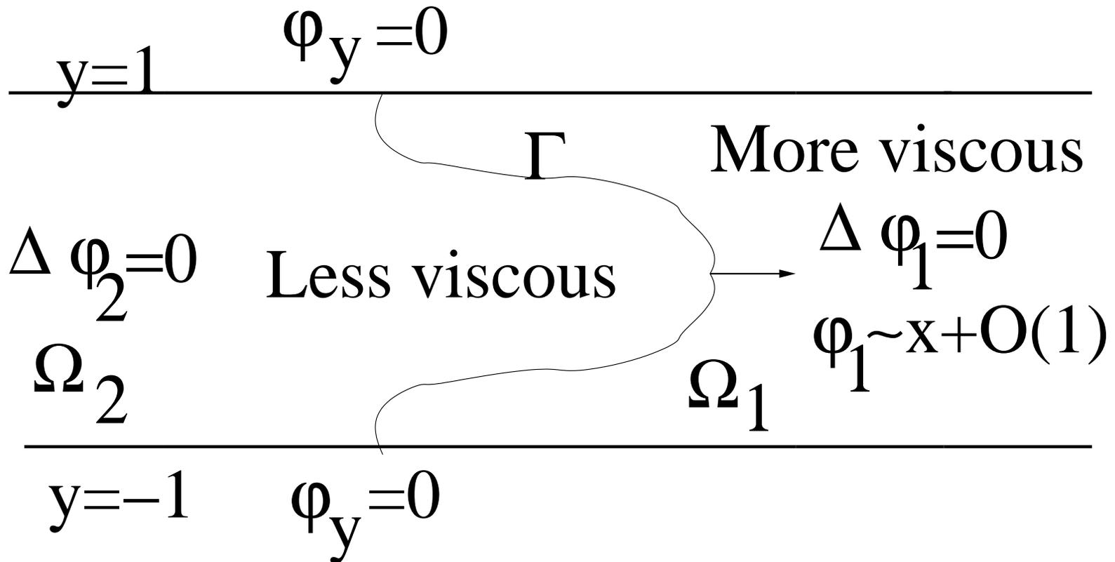
On  $\Gamma$ ,  $\phi_1 - \frac{\mu_2}{\mu_1} \phi_2 = \epsilon \kappa$ ,  $\frac{\partial \phi_1}{\partial n} = \frac{\partial \phi_2}{\partial n} = v_n$ , normal interface speed
