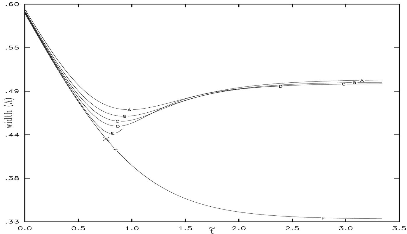
**Evolution of "finger width"  $\Lambda = 1/\text{tip speed}$  for a sequence of decreasing  $\epsilon$ . Prediction based on formal asymptotics agree with numerical computation (Siegel *et al*, 96)**
