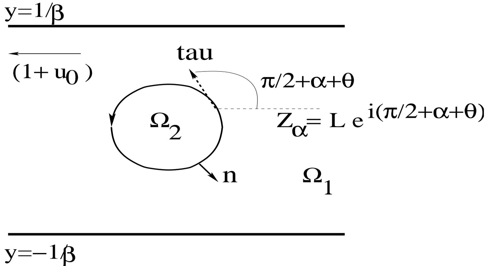
Hele–Shaw Bubble evolution in the frame of the steady bubble.
