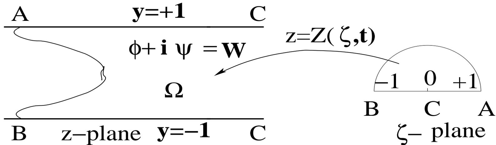
**Conformal map from unit-semi-circle to physical domain  $\Omega$  in one fluid problem**
