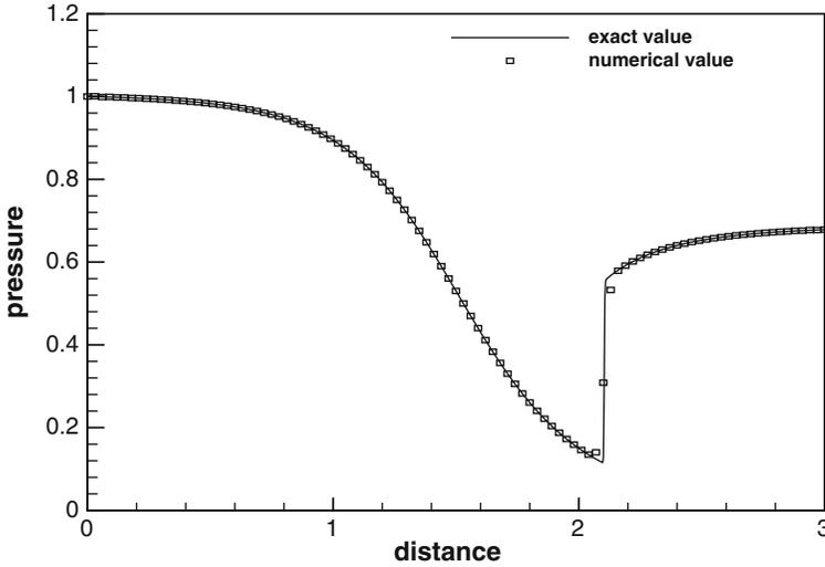
Fig. 4. Steady state pressure for the nozzle flow.
