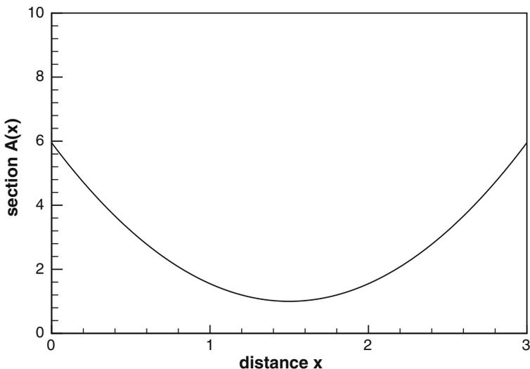
Fig. 3. The shape of a convergent-divergent nozzle.
