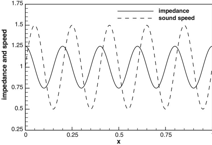
Fig. 1. The impedance  $Z(x)$  and the sound speed  $c(x)$  for the smooth media.
