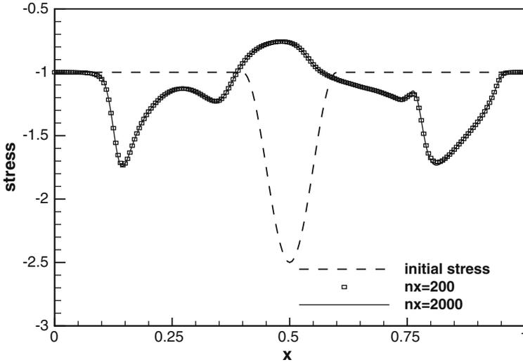
Fig. 2. The numerical (symbols) and the “exact” reference (solid line) stress  $\sigma(x)$  at time  $t = 0.4$  s.
